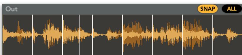
The current output waveform (the sum of all main and x-syn components) is displayed in yellow, with the left channel waveform displayed in bright yellow and the right channel in dark yellow.
