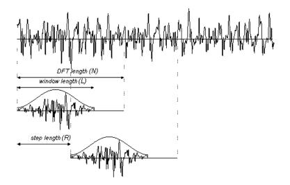
Figure 2.1: Signal windowing and Short Time Fourier Transform parameters.
