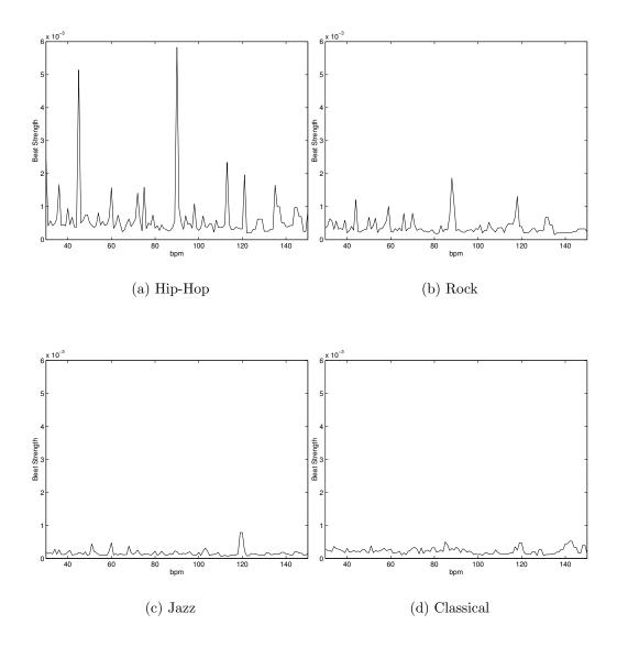
Figure 5.10: Beat histogram examples. High peaks correspond to high beat strength. Peaks separated by integer bpm multiples denote rhythm regularity.
