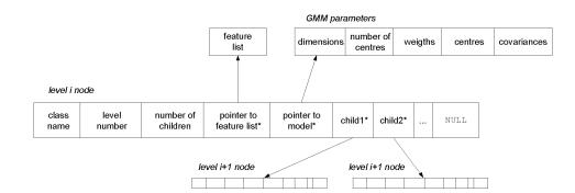
Figure 8.2: Implementation of a tree node. Asterisks denote pointers.
