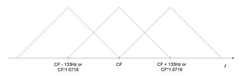
Figure 5.3: Definition of the MFCC filterbank. CF = Center Frequency (from [37]).
