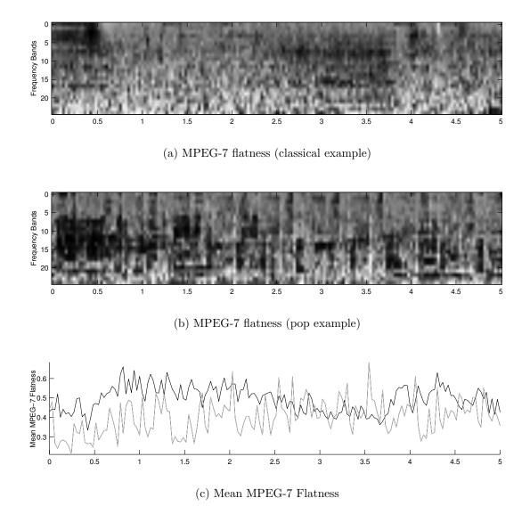
Figure 5.6: MPEG-7 flatness and mean flatness from the examples plotted in Figs. 5.1(a) and 5.1(b).
